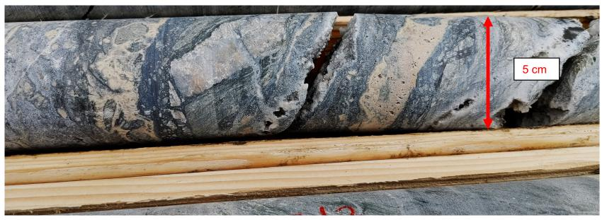
Figure 2. California Lake Zone core photo – multi-stage cross-cutting hydrothermal breccia. Darker areas contain fine grained sulphides including sphalerite, galena, tetrahedrite and arsenopyrite. Fractures, outside of breccia are also sulphide-bearing.
