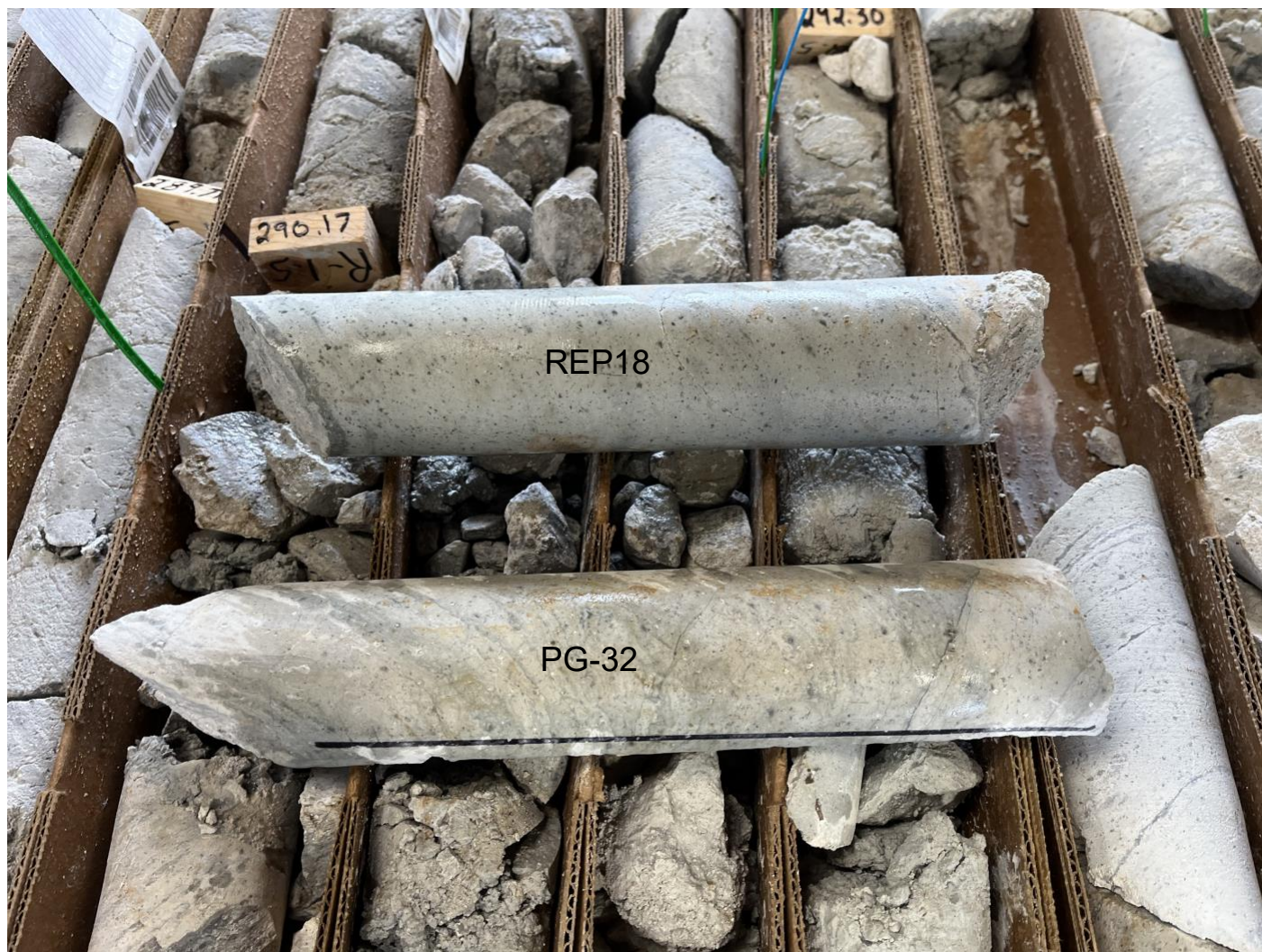
Figure 4. Photo of Altered Rhyolite Drill Core – REP 18 (top) and PG 36C (below) laying on box from REP 18
