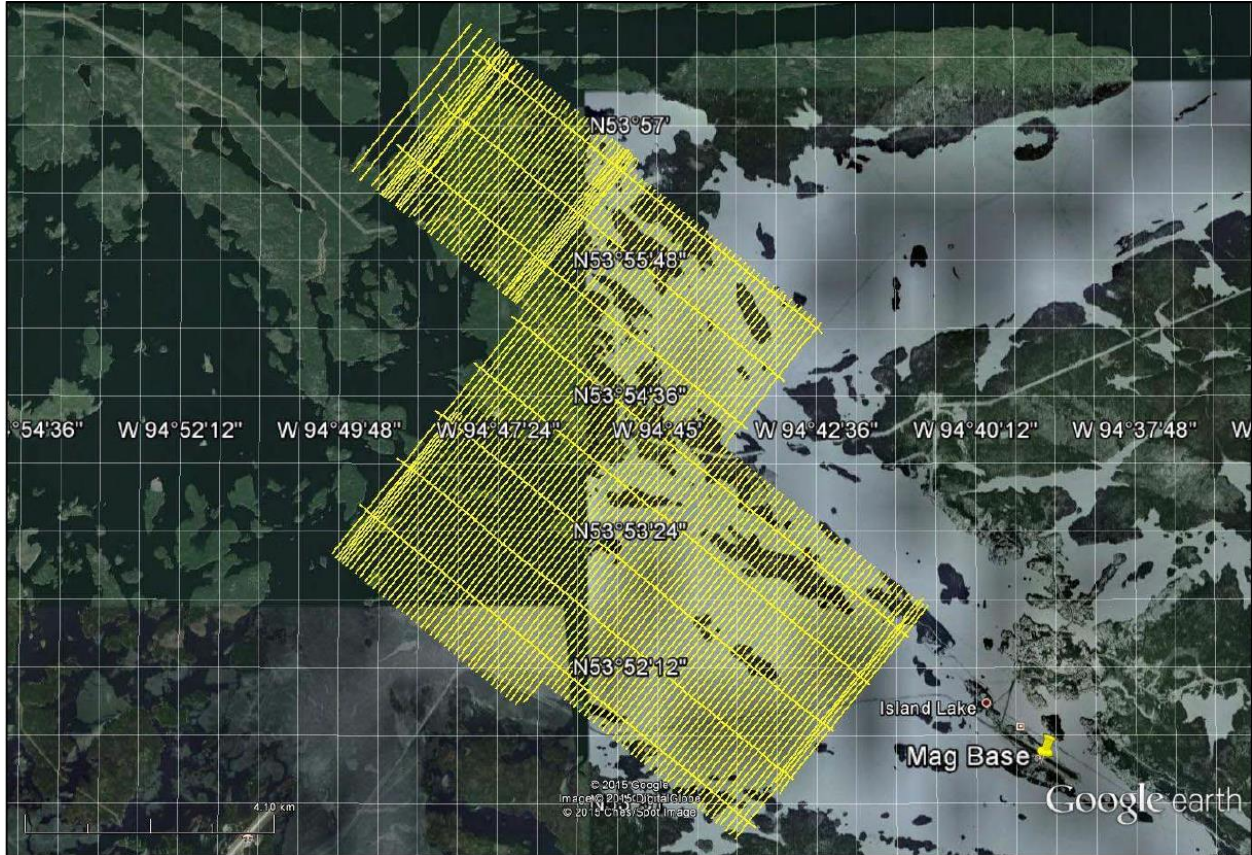
FIGURE 9.1 AIRBORNE VTEM AND MAGNETIC SURVEY FLIGHT LINES ON GOOGLE EARTH IMAGE
