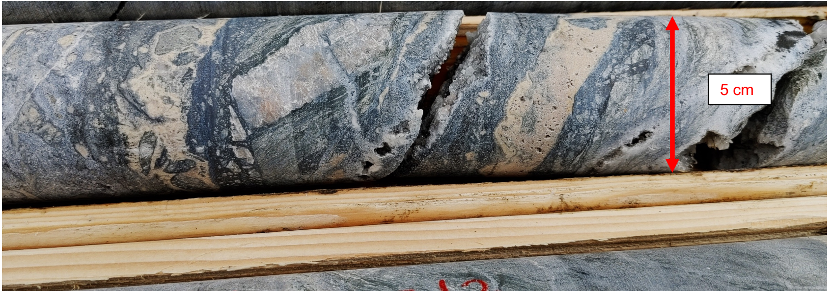
Figure 2. California Lake Zone core photo – multi-stage cross-cutting hydrothermal breccia. Darker areas contain fine grained sulphides including sphalerite, galena, tetrahedrite and arsenopyrite. Fractures, outside of breccia are also sulphide-bearing.
