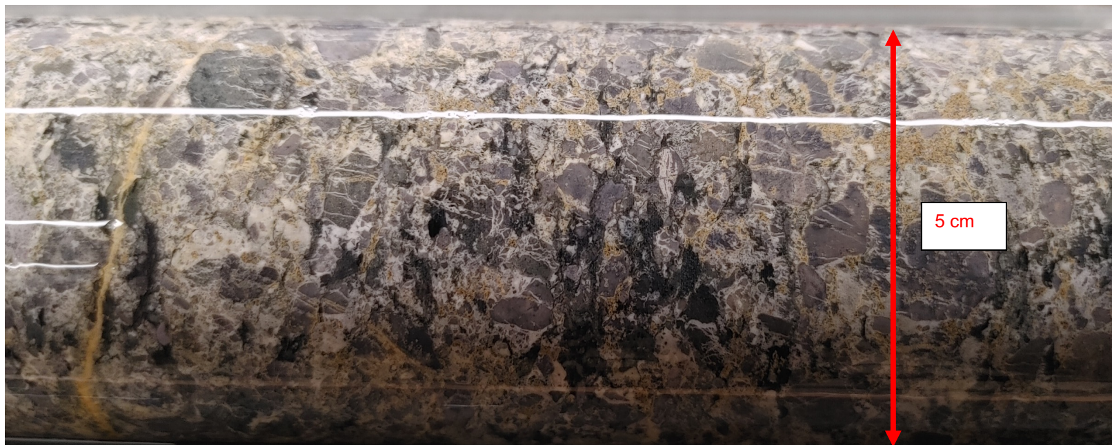
Figure 1. Big Silver Core photo – sedimentary breccia with silicified clasts and 10-15% light brown sphaerite (zinc mineralization)
