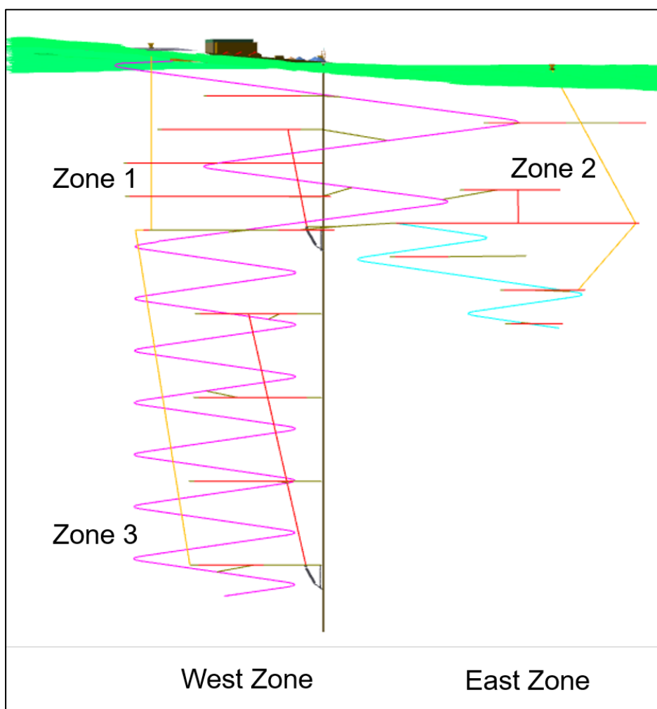
Figure 16.1 Pickett Mountain Mine Design Longitudinal Section Looking North
