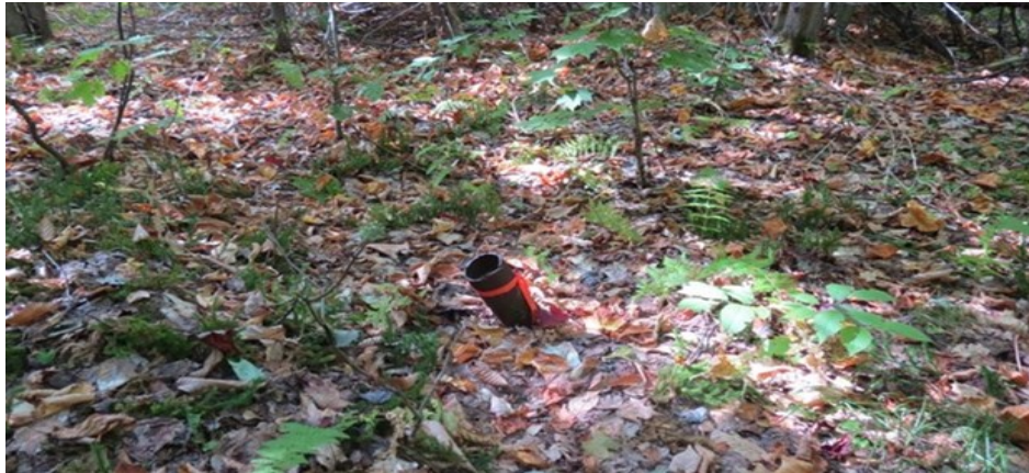
Figure 12.3 The casing located in the field and identified as being the collar for hole 66-46
