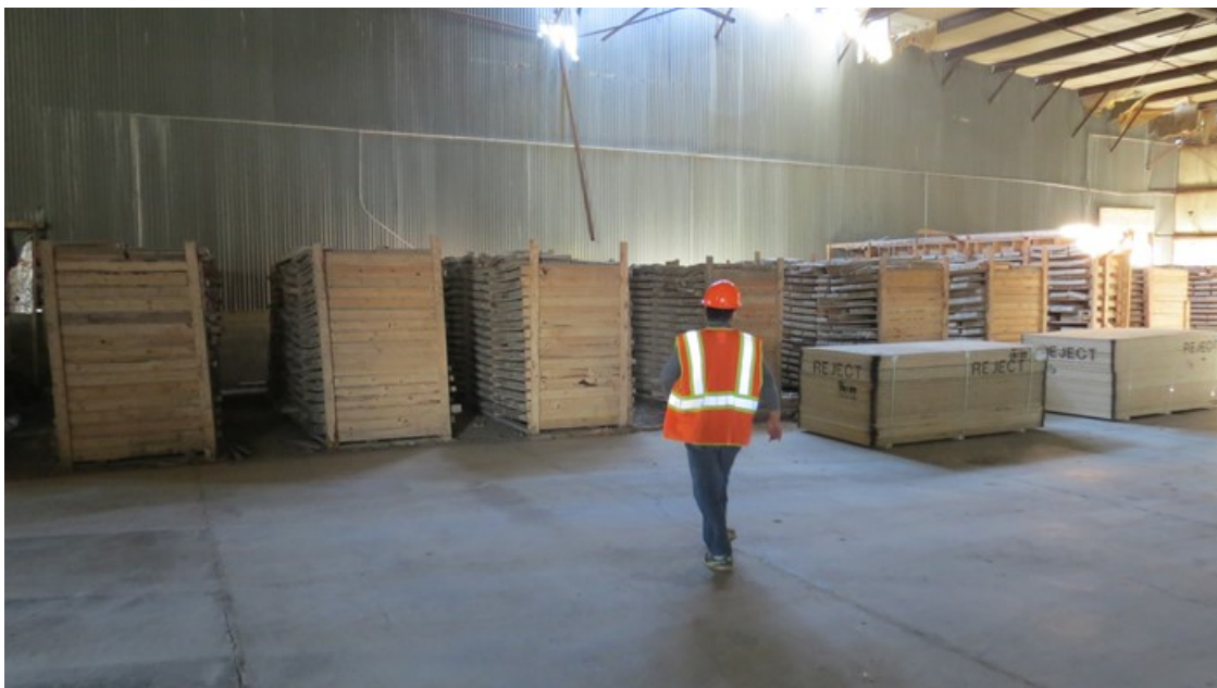
Figure 12.1 Core storage facilities maintained by Huber Engineered Woods at their plant located in Easton, Maine at “remote warehouse 1” where a majority of the core is stored piled on shelving units
